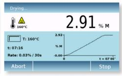
Drying cycle page with graph, with parameters
