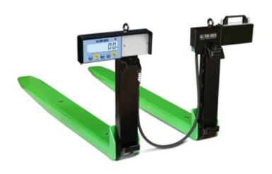
Pair of forks with an integrated weighing system for lift trucks, easy to use, sturdy, and reliable. The optional wireless indicator to install in the cabin makes weighing operations easier and has a large range of accessories. Operates by a rechargeable battery or directly powered from the lift truck. Compatible with any lift truck having a DIN 15173 - FEM fork holder plate, of the IIA (IIB optional) or IIIA class. Available in CE-M approved version.
